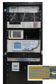
Primary Voltage Standard used to define the “Volt” Image Courtesy of NIST and Hypres Inc.
