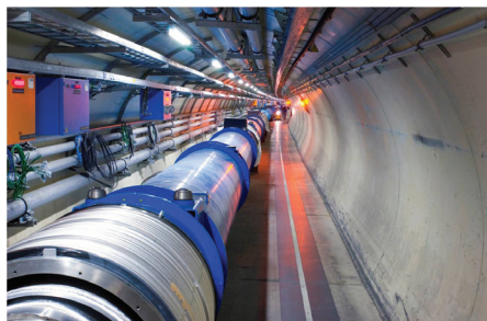
Accelerator Magnets fully operational in the LHC Tunnel Image courtesy of CERN, Geneva
